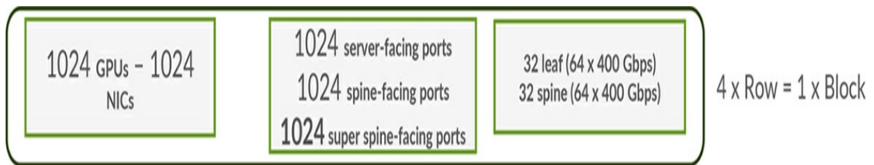
Figure 3-11 GPU scale supportability per block with five-stage Clos fabric
