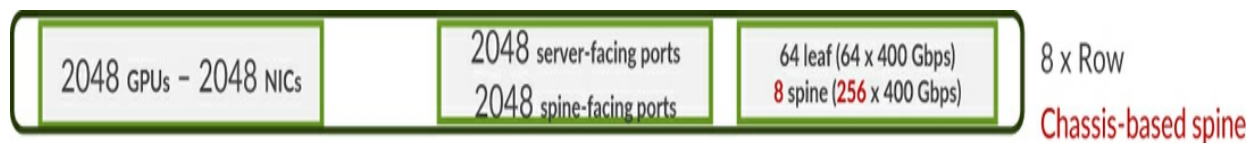
Figure 3-10 GPU scale supportability with a chassis-based spine
