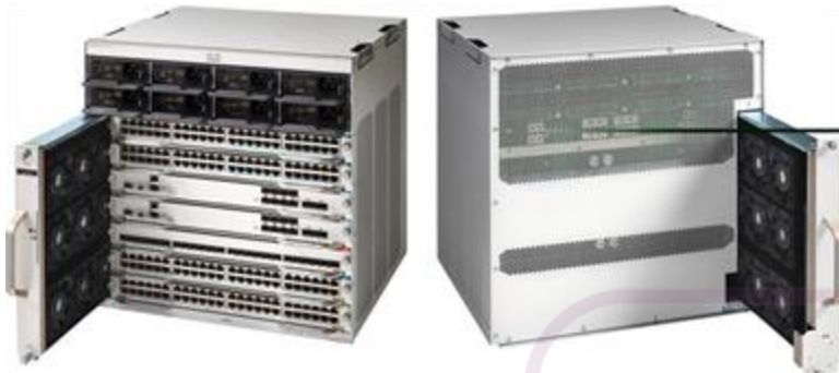
Figure 2. Dual serviceable fan tray
