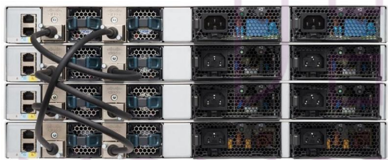
Figure 4. Cisco Catalyst 9200 Series Switch stacked units
